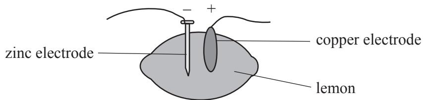
In an experiment to determine the e.m.f. and internal resistance of a battery made from three lemon cells, a student measures the current  $I$  for different potential differences  $V$ . Her results are shown below.
